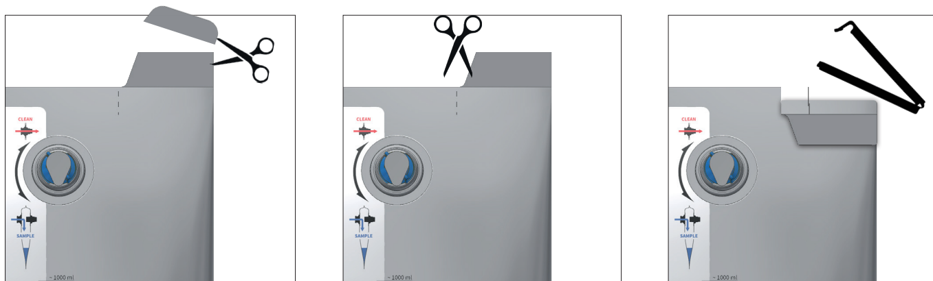
PICTURE 15. Retrieving sample from the KEOFITT Sampling Bag™ by cutting the foil. After pouring out the sample from the opening made by a pair of scissors or the like, the area for folding/closure can be extended by cutting the dotted line.
