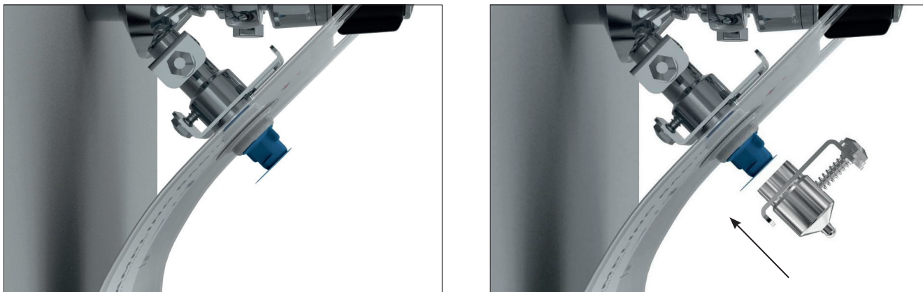
PICTURE 9. Left: Protecting aluminium foil on the outlet. Right: If no cleaning, disinfecting, or sterilization of the flow path is necessary, the Quick Coupling KSB Outlet stainless steel plug can advantageously be mounted to support the foil when sampling.
